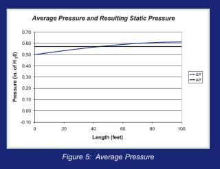
If the ISP and SPR are added and FL subtracted, the resulting number will be the accumulated static pressure at the endcap. In most cases, the maximum static pressure of the system.
