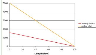
Velocity and Airflow along Duct Length
