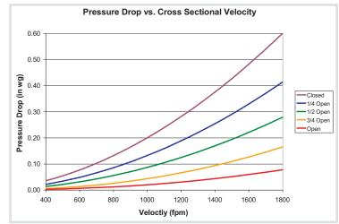
Fig. 4: Pressure drop vs. velocity
