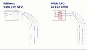
Figure 7: Reduces Turbulence
