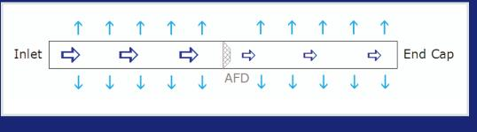
Fig. 9: AFD resists inflation velocity, resulting in smoother start-ups.
